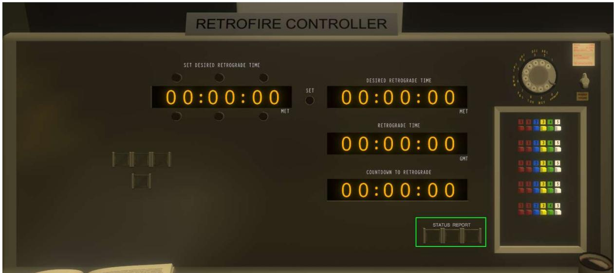
The Retrofire Controller desk has indicators to set the desired retrograde time, see the currently planned time, when it will happen in GMT timezone, and a countdown to it. In addition, indicators show if the retrograde jettison squib is armed, and if each of the retrograde rockets (3x) fires.
