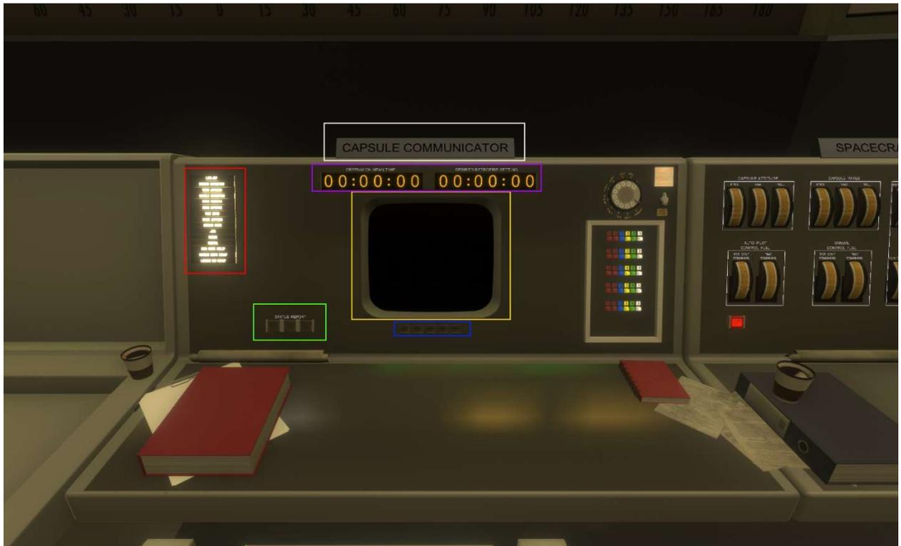
The CAPCOM is in charge of communicating with the capsule. Realistically, CAPCOM is the only person directly communicating with the capsule, everyone else talks to the capsule through them. CAPCOM can see the current progress of the flight, as well as having a monitor for seeing the launch-pad.
