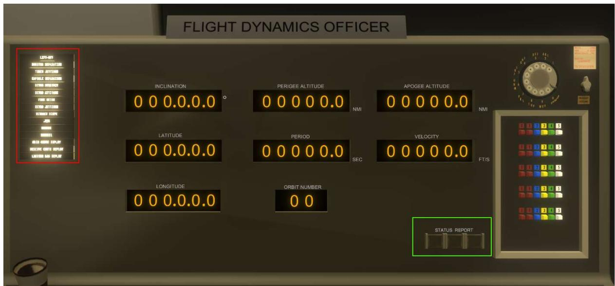
FIDO is in charge of monitoring the orbital parameters of the spacecraft. The desk has the familiar sequencer to show the state of the mission, as well as indicators for the current orbital inclination, perigee and apogee altitude, the latitude and longitude to know the current location of the spacecraft above Earth (as seen on the map), the orbital period (in seconds), current velocity and the orbit number.
